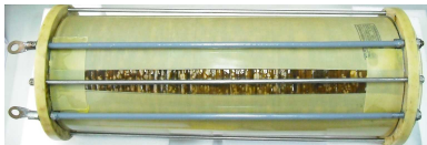
Fig. 3. The 0.2H HTS coil developed by Innopower and CASEE
